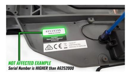
For example, on this model serial number A6252000 and lower are affected products.
