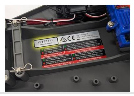
How to Identify an Affected Model by Serial Number Range
